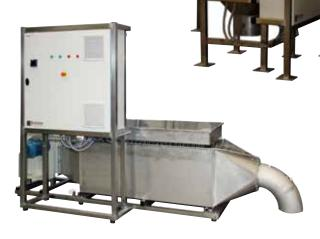
Horizontal air direction 120kW Power: Voltage: 3x400V
