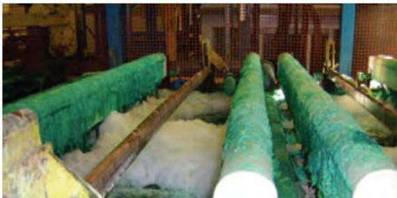
Air agitation showing foam, and contamination of tank and other surfaces
